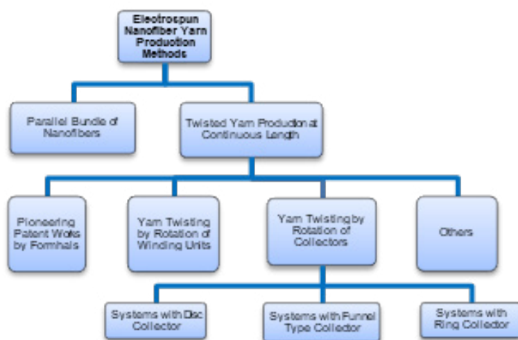
Figure 1. Classification of electrospun nanofiber yarn production methods in general
