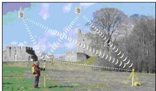
Figure 15. By DGPS techniques, real-time kinematic observation data is transmitted to rovers by telemetry
