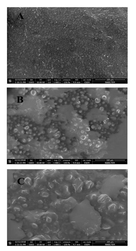
Fig 3 Micrographs of the emulsions prepared with egg yolk (a), whole egg (b) and egg white (c) powder
