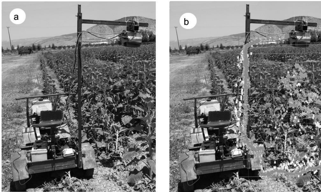
Figure 1. The vehicle with the vertical and horizontal mast carrying the laser scanner (lidar) (left) and the alignment of measurements (right).
