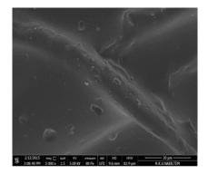
Figure 2b. SEM images of Cu (I)O <5µm particles on cotton by using concentrations of 1%.
