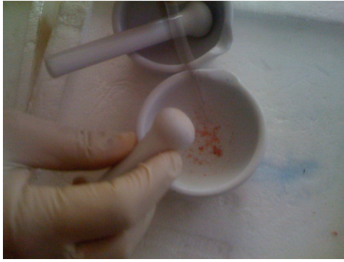
FIGURE 2: Mechanical disruption of the tissue which is frozen in the presence of liquid nitrogen.
