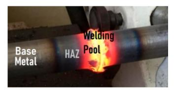
Figure 1. Air-cooled rotary inertia friction welded steel-steel rod.
