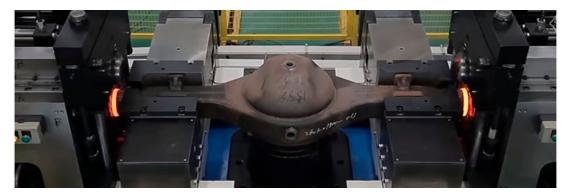
Figure 11. Friction welding of axles (China RCM).
