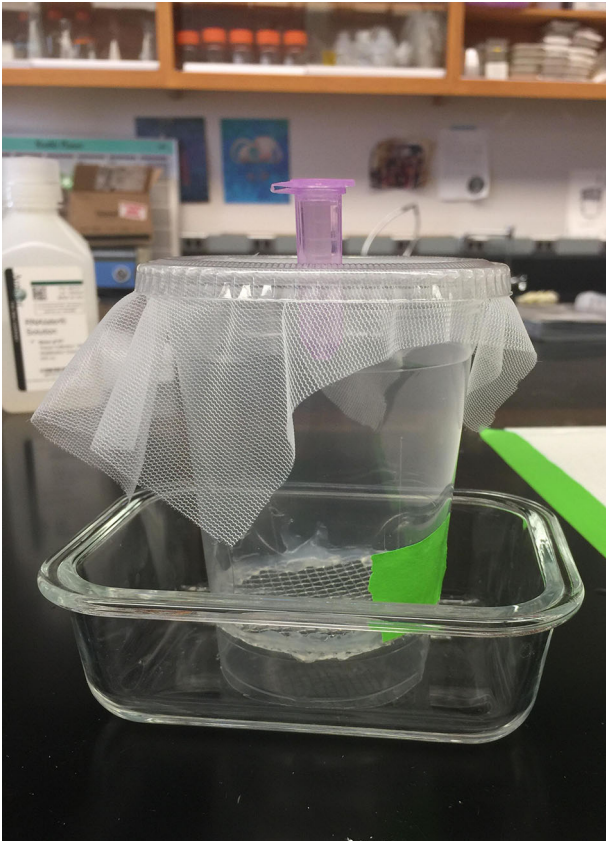
Figure 4. Modifying a Solo Cup® rearing cage to collect wax scales by inserting a wire mesh false floor, removing the bottom of the cup, and placing over dish. Photos: O’Grady M.
