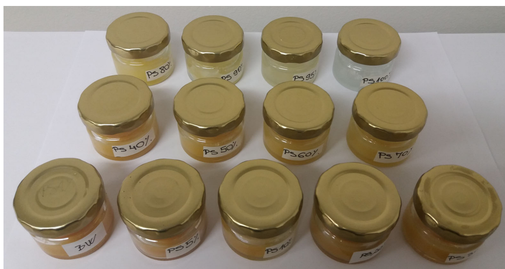
Figure 47. Containers with prepared adulterant (paraffin/paraffinum solidum – PS)–beeswax mixtures after melting. Photo: Svečnjak L.
