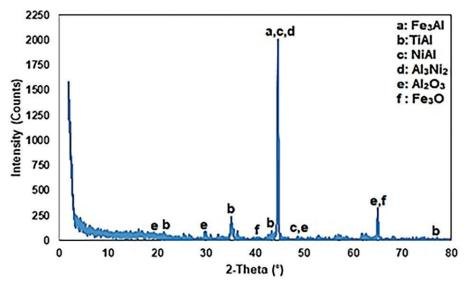
FIGURE 3. XRD graph of S3 sample.
