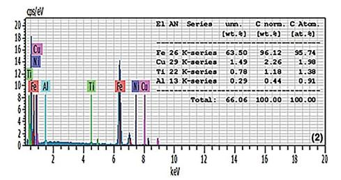
FIGURE 2. EDX analysis results of S5 sample.
