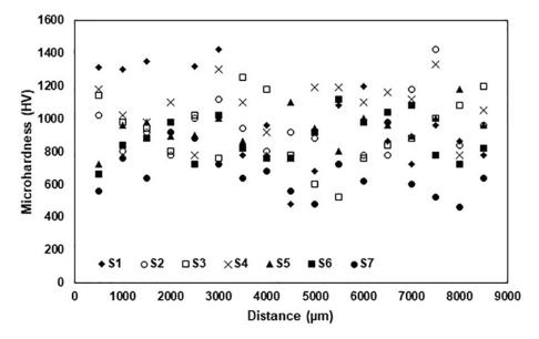
FIGURE 5. Variation of microhardness values of S1-S7 samples.
