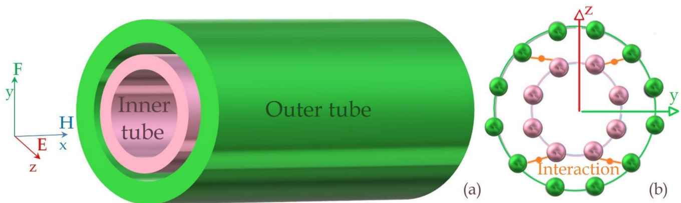
Figure 1. (a) EM wave propagation in the DWCNT, (b) EM interaction between DWCNT's inner and outer tubes.
