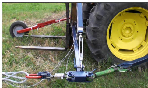
Fig. 4. Purpose-designed drawbar mechanism with a converted forklift.
