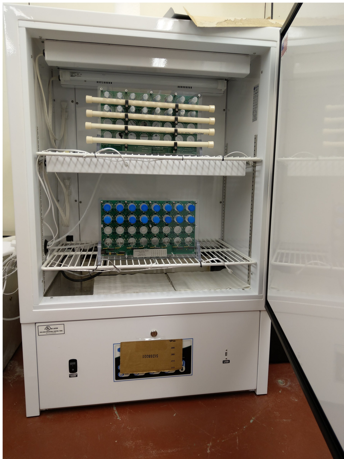
Fig 3. Monitor system in incubator. Top rack shows the monitor with CPVC piping which allows water or treatment access for the bees. Lower rack shows falcon tube caps containing bee candy.
