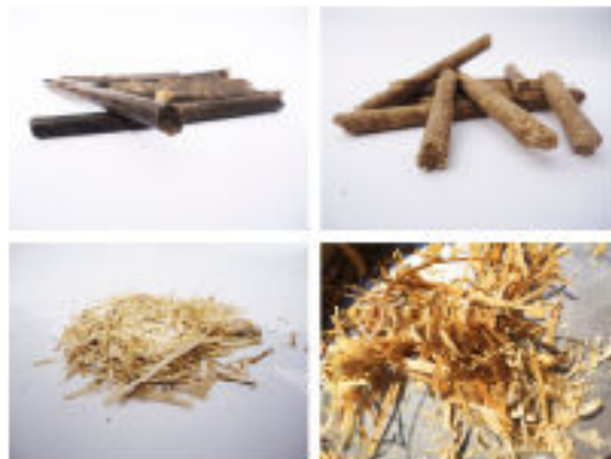
Figure 2. Some of the feedstocks: pellets and natural fibres used in experiments, 1. Canola stalk pellet, 2. molasses pellet 3. Natural fibre, 4. Wood fibre, (From left to right in rows) Photography by Esen Gökçe Özdamar, 2016
