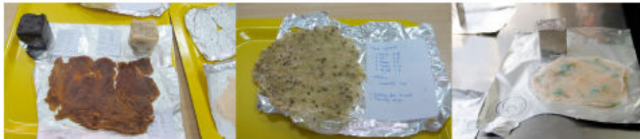
Fig. 4. Bioplastic cubes and sheets made of basic ingredients such as potato starch, vinegar, glycerin, water, salt with additives coffee, pine needles, camomile, chilli pepper, cotton and beeswax, cooked between and 3,4-6,20 minutes, baked at 60°C for at least 2 hours, from left to right, Photos by Esen Gökçe Özdamar and Julia Janku
