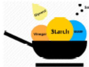
Figure 1. Basic ingredients of bioplastic and heating in an oven, just below boiling 95°C.
