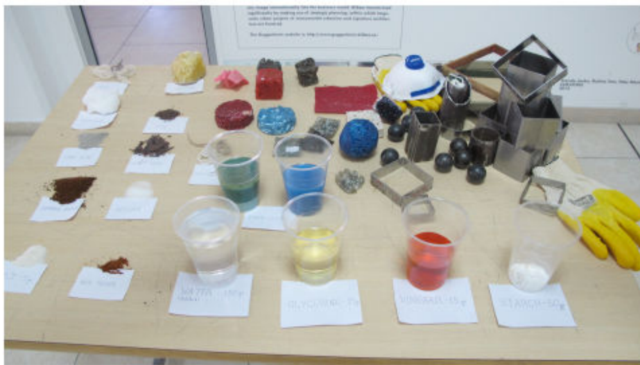
Fig. 18. Basic ingredients of bioplastic and additives used, Photo by Esen Gökçe Özdamar
