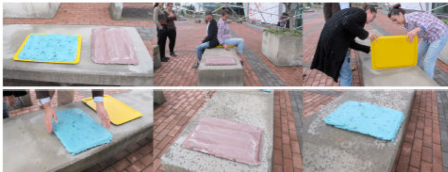
Fig. 20. Bioplastic tiles left for drying open-air for observation, Photos by Esen Gökçe Özdamar
