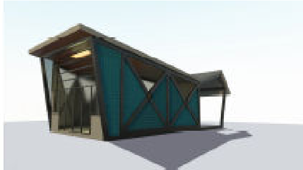
Figure 9. A close view to bioplastic facade, Tekirdag, Turkey, 2016 Rendering by students Burak Saral and Selin Koca
