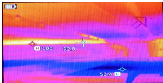
Figure 4. Thermal camera view of fabric inside the chamber
