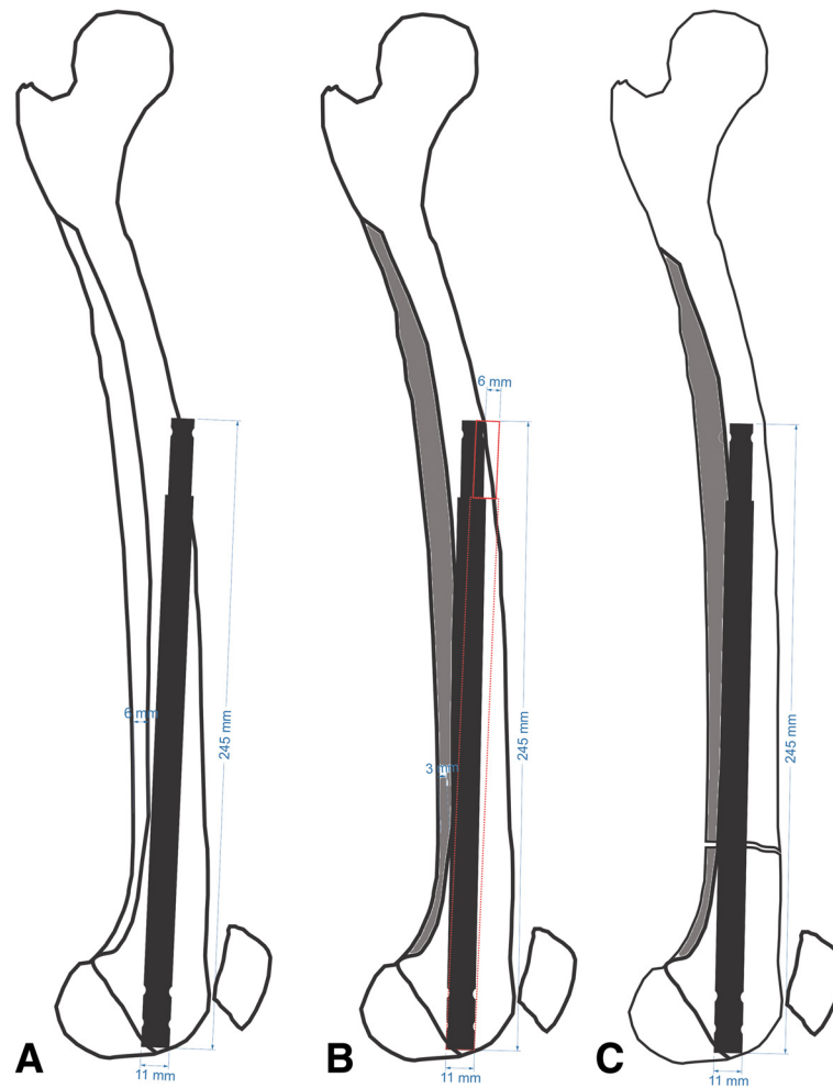
Fig. 7 a A 6-mm protrusion of the nail tip on the anterior cortex in an unreamed application with a straight nail. b A 6-m posterior displacement of the nail tip after 3 mm of reaming 10 cm proximal to the intercondylar notch. c Greater than 6 mm posterior displacement of the nail in an osteotomized femur
