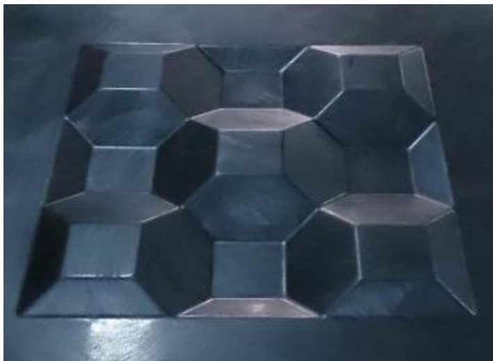
Fig. 2. The lacquer coated mold for the core.
