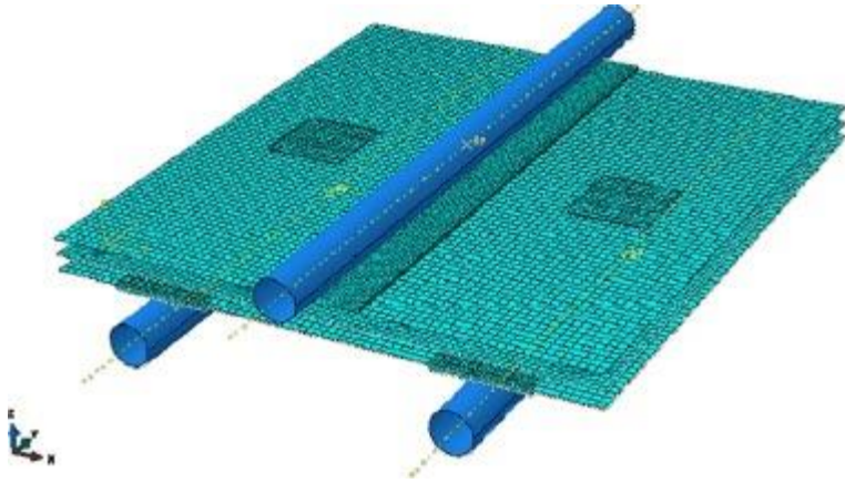
Fig. 9. FE model of three-point bending and meshed assembly.
