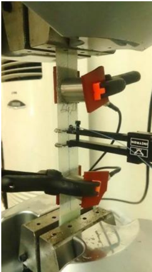
Fig. 3. The tension test setup.
