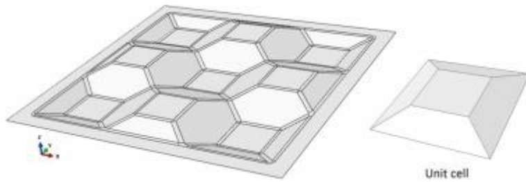
Fig. 1. The schematic representation of the core design introduced in this study and unit cell.
