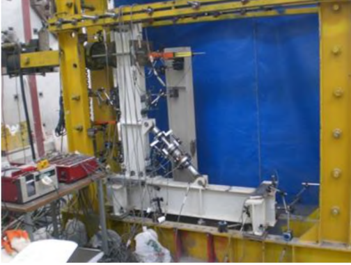
Figure 3 Cyclic steel beam-column connection tests, [14].
