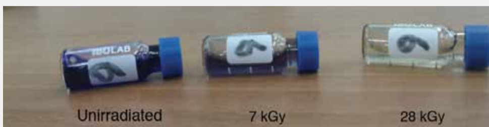
Figure 3. The resulting color change in crystal violet-polymer gel dosimeter following irradiation
