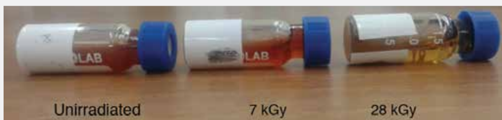
Figure 4. The resulting color change in methyl orange-polymer gel dosimeter upon irradiation
