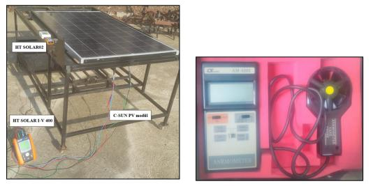
Figure 4. PV module and devices used during measurement
