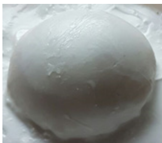
Figure 3. The top view of PDMS coated SH-P.
