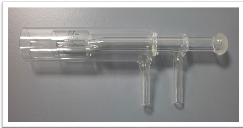
Şekil 2.14. Torch örneği ( https://commons.wikimedia.org/wiki/File:ICP_quartz_torch_3.JPG )
