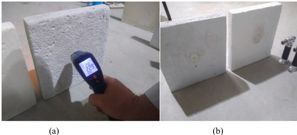
Fig. 12. (a) Back surface temperature measurement of foam concretes exposed to a temperature of about 1200 °C (b) The appearance of the samples after the experiment.
