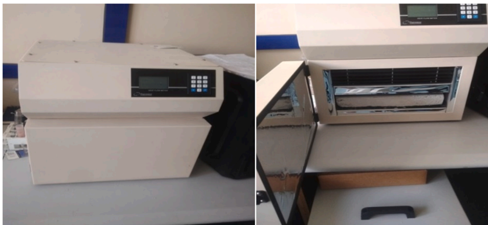
Fig. 5. Test tool used to determine the thermal conductivity coefficient.
