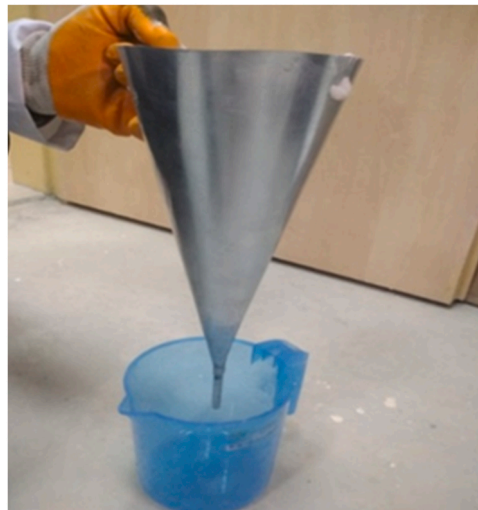
Fig. 3. Determination of consistency of foam concrete with The Marsh Cone Flow Test.
