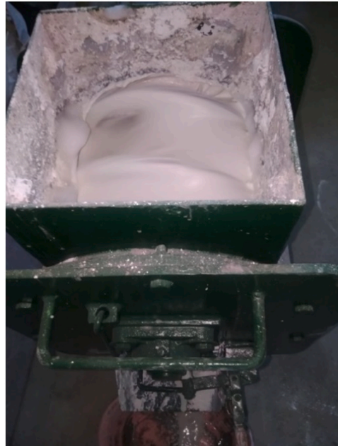
Fig. 1. Helical type mixer used in mixing foam concrete.
