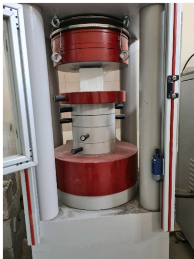
Fig. 4. Test equipment for compressive strength test.
