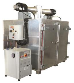
Figure 2. Heat treatment (sterilization) machine developed by Riverm Company, Turkey.
