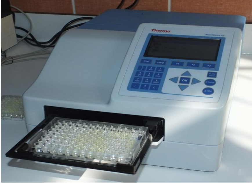
Şekil 3.2. Thermo Scientific Multiskan FC ELISA Plate Reader
